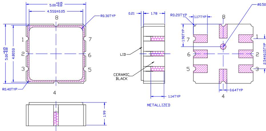
*Fig 10: Soldering Device Outline*
