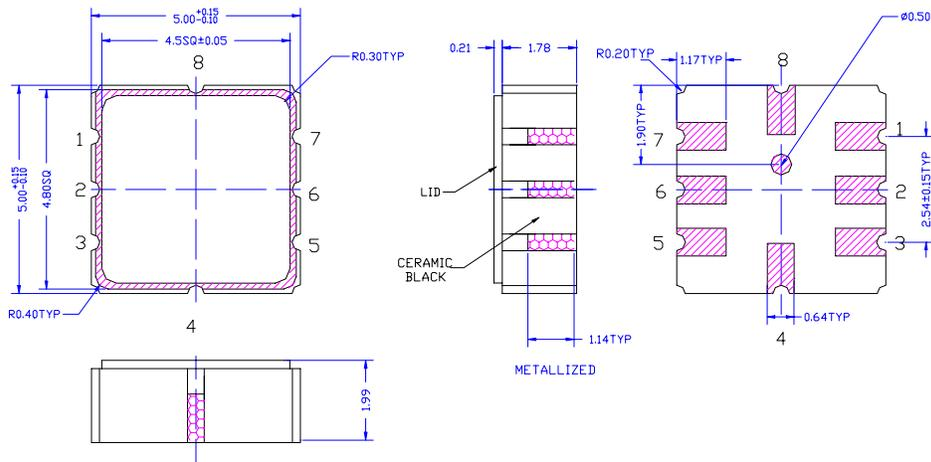
*Fig 10: Soldering Device Outline*
