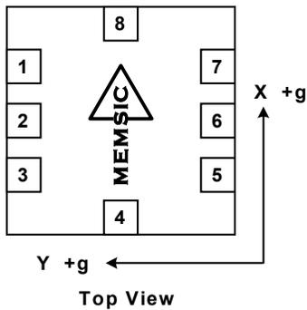
**Note:** The MEMSIC logo's arrow indicates the +X sensing direction of the device. The +Y sensing direction is rotated 90° away from the +X direction.
